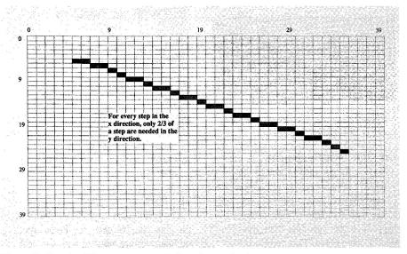
Figure 3. X and y differences unequal; line shows aliasing.
