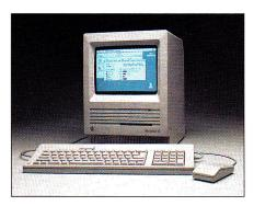
The Mac's Standard Keyboard, shown above, is also compatible with the GS, thanks to the ADB protocol. (Photo courtesy of Apple Computer.)
